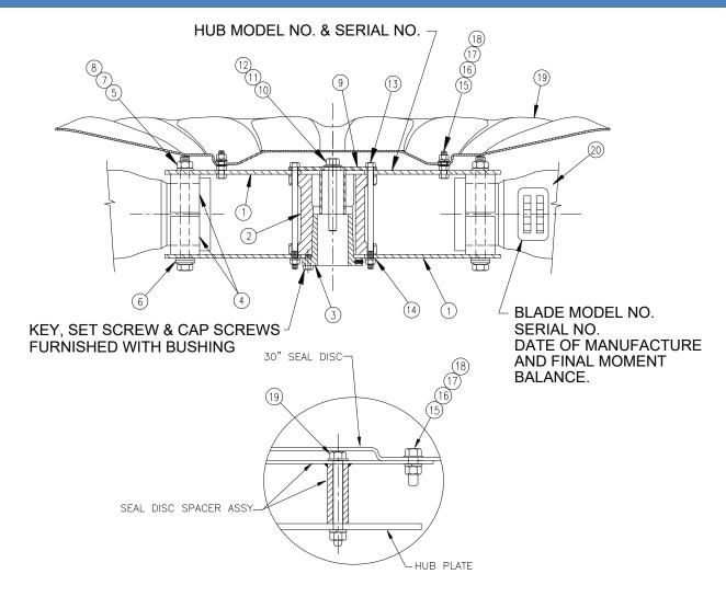
Seal Disc Spacer Mounting for 5H HUB ASSY, 4-8 BLADES
